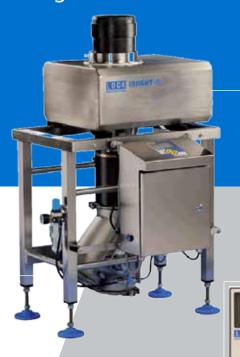
sensitivity offer the ideal solution for detection and rejection of metallic contaminants during the handling of free falling product. Ideal for processing cereals, cocoa, coffee, sugars, spices, dried fruit and vegetables, flour, milk powder products, chemical granules, rice and plastic pellets.
